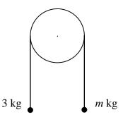
The particles have mass 3 kg and m kg, where m < 3. They are attached to the ends of a light inextensible string. The string passes over a smooth fixed pulley. The particles are held in position with the string taut and the hanging parts of the string vertical, as shown in Figure 1. The particles are then released from rest. The initial acceleration of each particle has magnitude  $\frac{3}{7}g$ . Find
